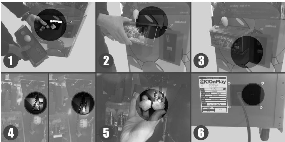
1. pass the cable of the module through the hole.
