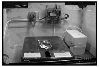
NOW OBSOLETE, TABLES PRODUCED UP TO END OF 2001. USES JOFEMAR TREMOYA T20b OR T21b TOTALISER MECH. POP CHANGED USING THE MECH DIP SWITCHES. BLACK, 12 VOLT MOTOR. IF PCB NEEDS REPLACING, MORE ECONOMIC TO UPGRADE TO SAMIK 4.
