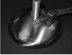
SAM tables are levelled in a simpler and easier fashion than traditional pool tables. The chrome/copper foot is secured to the long bolt by an alan key bolt. This bolt screws into the bottom of the leg. It has flats on it to accept a 13mm spanner. Adjusting this bolt is what raises and lowers the leg, **not spinning the foot.**
