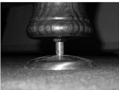
On installation the foot assembly should not be screwed right into the leg, or the flats will be hidden. Screw in half way and then level the table by spanner. The lock nut should then be tightened against the bottom of the leg to stop movement.
